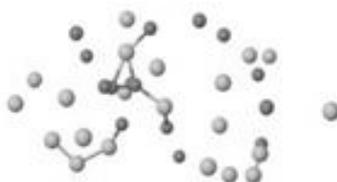
**Figure 5: The dispersing of initial 2KeV in 64 atoms supercell of SiC after 1000 steps at time step 0.1fs**
