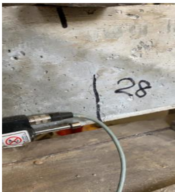
Figure 3: Electrical gauges used to measure stresses applied on the beam at location of failure
