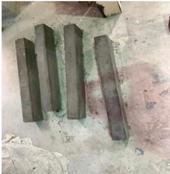
Figure 2: Concrete beams after being removed from wood molds
