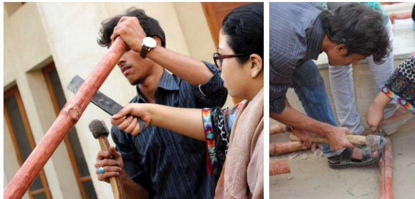
Figure 13 (a) (b): Basic Technique of Split Bamboo
